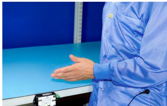
Snap for Wrist Strap Connection to Dedicated Ground Sleeve
