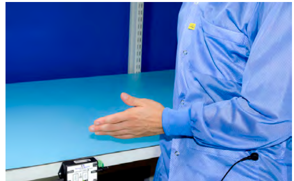
Snap for Wrist Strap Connection to Dedicated Ground Sleeve
